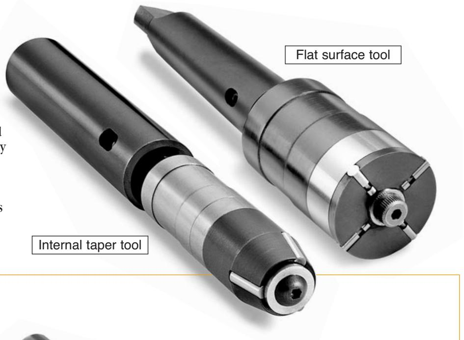
Where part size varies and surface finish is the primary requirement, expanders, contractors, and compensating tools produce consistently excellent surface finishes.
