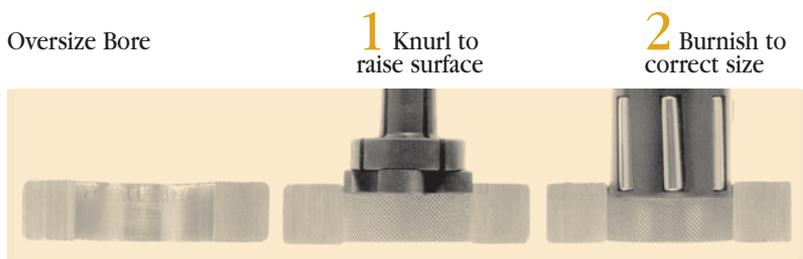
An oversize bore may be machined out-of-tolerance or made oversize by excessive wear. Here's how the KB Process can salvage this part:
