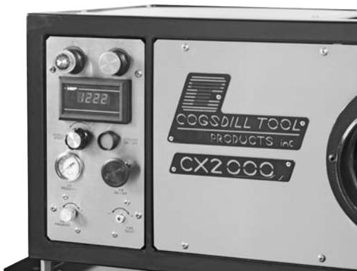
**Easy-access control panel is located on the front of the machine.**
